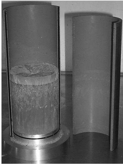
Figure 1. One hundred twenty-millimeter casting form with a solid block of ADN/Al. The separate layer on the top of the block is frothed, very low-density material due to ammonia release from ADN + MgO.
